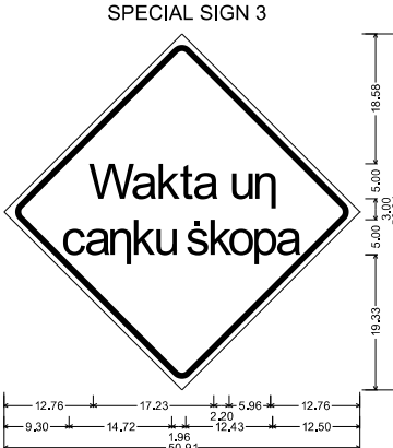
36.00" across sides 0.88" Border, 0.63" Indent, Black on Yellow: "Wakta un", Arial 70% spacing; "canku škopa", Arial 3% spacing
