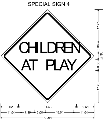
36.00" across sides 0.88" Border, 0.63" Indent, Black on Yellow: "CHILDREN", C 2K; "AT PLAY", C 2K 80% spacing;
